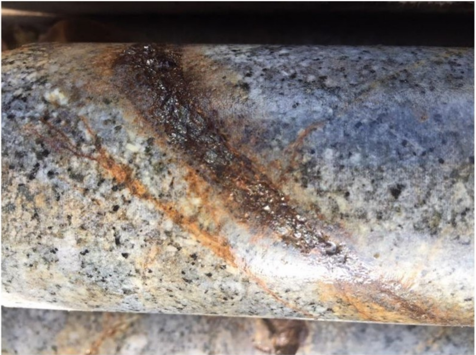
Quartz-pyrite-molybdenite-FeOx vein with probable bornite in the halo. KEX 19-004 @ 9.45 m. Note cross-cutting veinlets.
