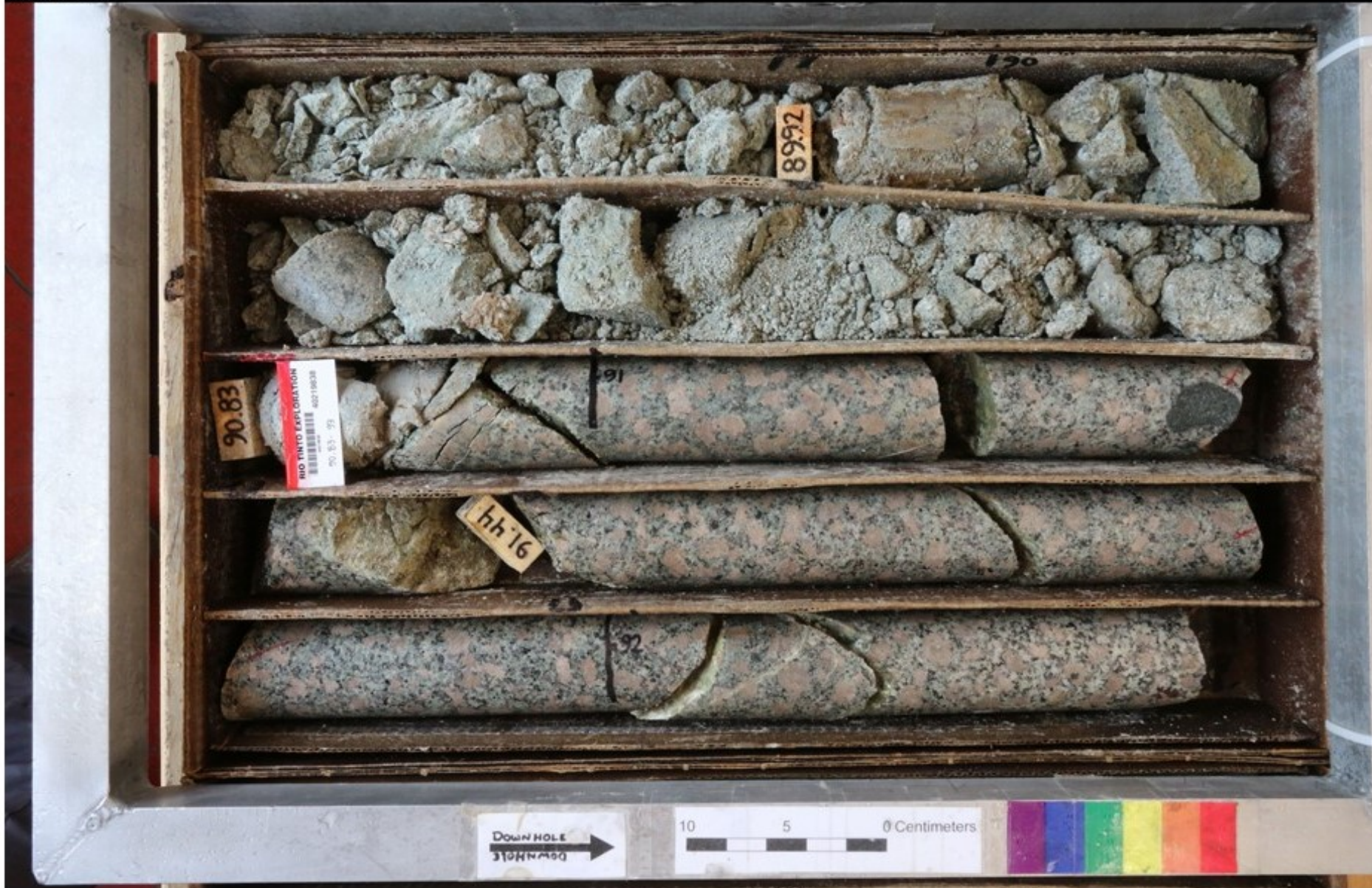
KEX 19-004 89.86-92.33. Fault zone above and megacrystic monzo-granite. Logged as clay alteration and sericitic alteration.
