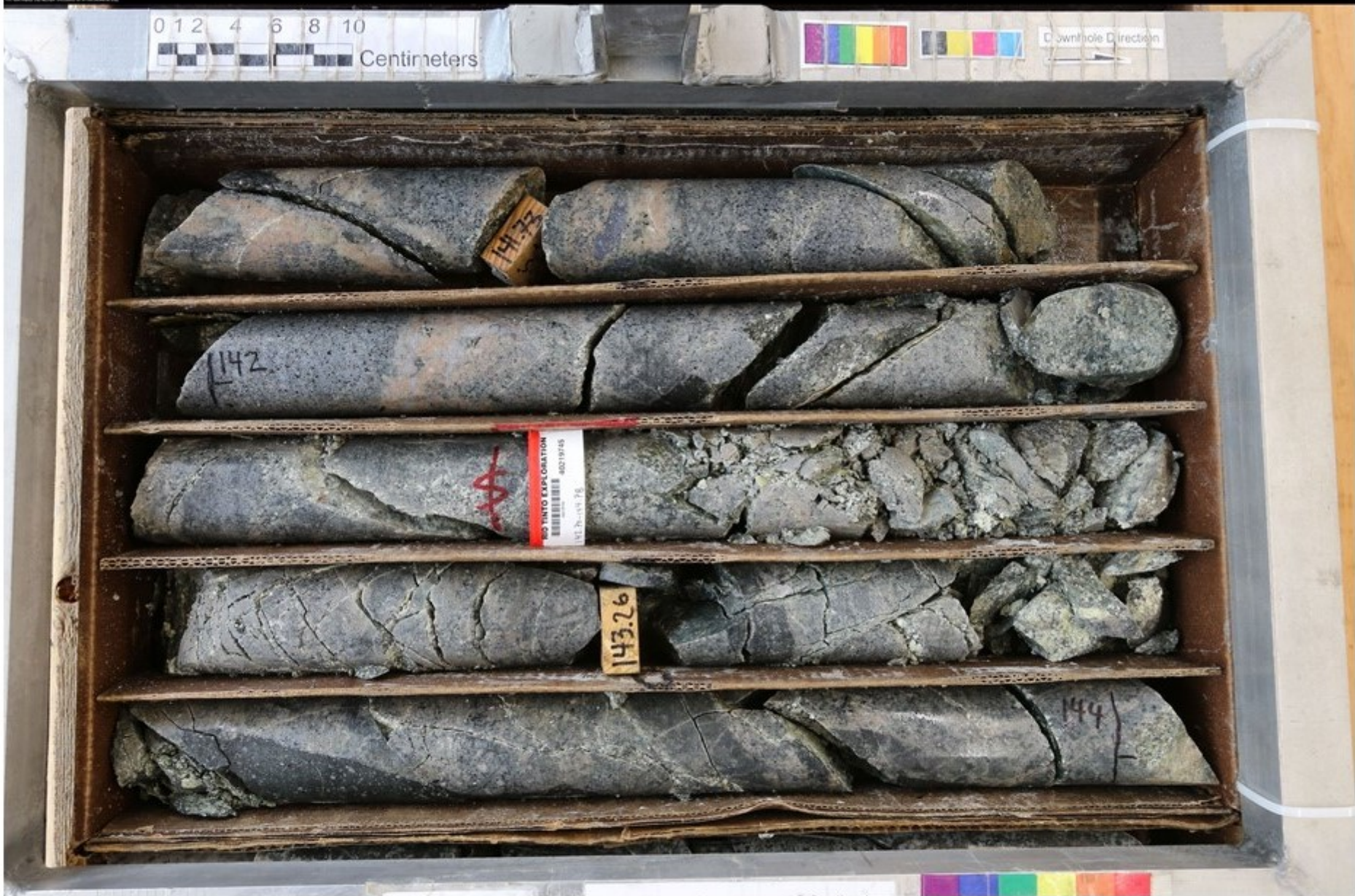
KEX 19-003A 141.57-144.04. Granodiorite, logged as potassic alteration. Note k-spar banding/veins.
