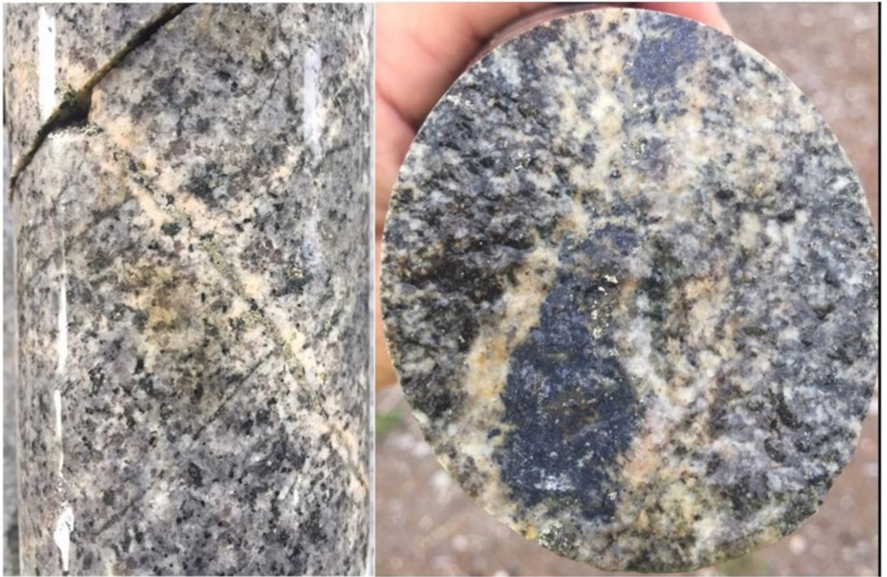
Quartz-pyrite-molybdenite-chalcopyrite +/- magnetite veins with K-feldspar halo @ 143.4 m. in KEX 19-001
