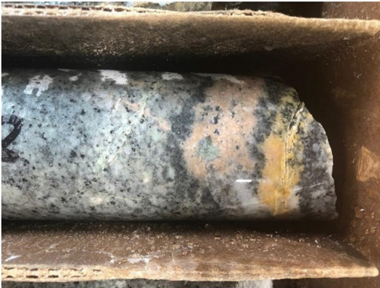
Quartz-kspars vein with molybdenite, pyrite, magnetite and chalcopyrite. Shreddy biotite halo surrounding the vein. KEX 19-003A @ 92.1 m.
