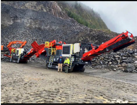
2022 Sandvik QH332 ..... #80-33203 260 Hrs, Mobile Cone Crusher, CAT C-9, 8” Feed Size, 220 MTPH, 6.5 Yd Feeder Chehalis, WA ..... $679,500
