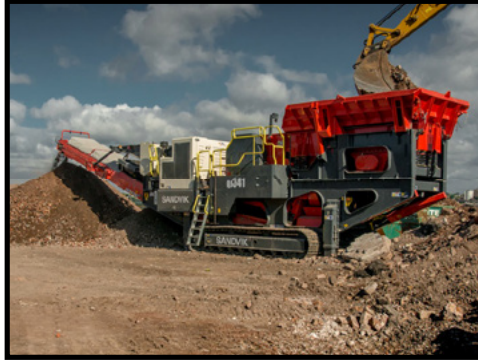
2022 Sandvik QJ341 ..... #80-34101 610 Hrs, Mobile Jaw Crusher, Tracked, Single Toggle C12 Jaw, 39” Conveyor Chehalis, WA ..... $639,500
