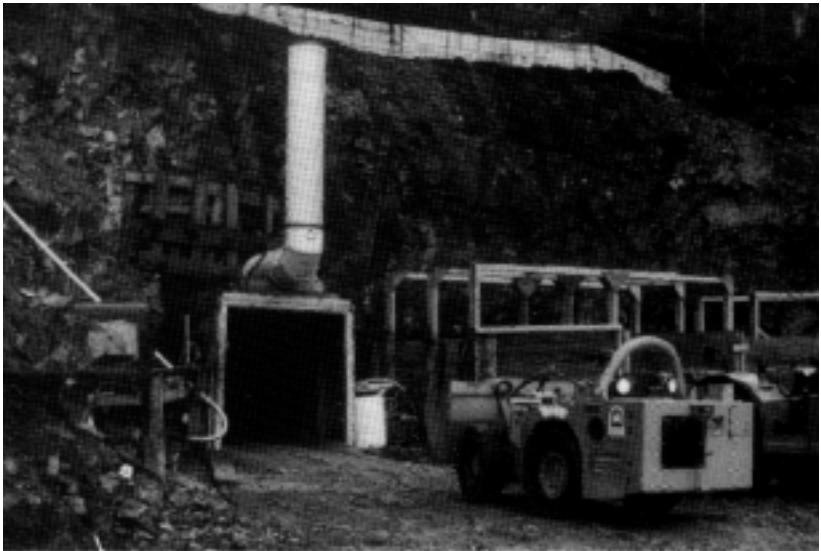
Collar of one of two bulk sampling adits, Quartz Hill molybdenum deposit (1981).
