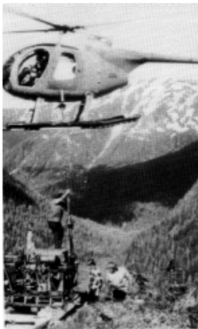
A helicopter slings an exploration drill into place at Quartz Hill in 1975
